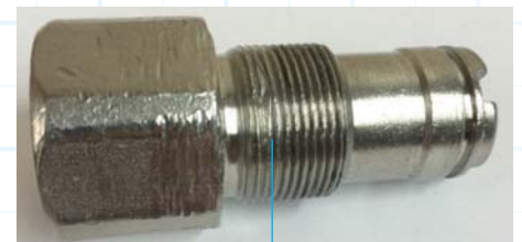
Damage to threads on SDX III Nozzle
